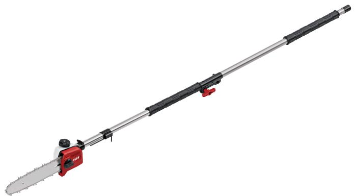
The pruner attachment (including 80 cm extension) for the battery-powered basic drive allows you to cut high branches to length without needing a ladder. Attachment can be mounted without tools. Thanks to the 25 cm long blade and a chain speed of 13 m/s, branches up to around 20 cm in diameter can be sawn off with ease. There is an automatic lubrication system with an oil reservoir (120 ml) on the pruner to keep the chain running smoothly.
